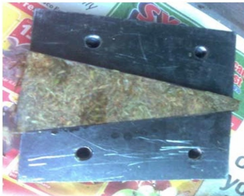
Fig. 6. Fabricated banana leaves-polyester-MEKP pyramidal microwave absorber in pyramidal mould
